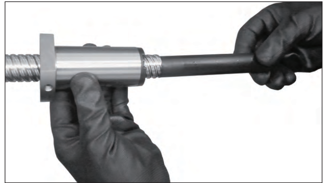
(4) Ensure that the ball nut is fully inserted before remove the mandrel.
