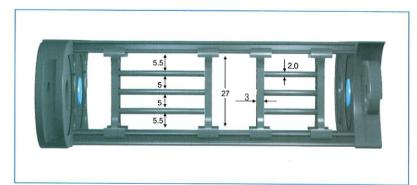
Dividers & Separator are differently installed into the inside of cable chain depending on number & size of cable and inside space of cable chain can be divided into max.4 story by separator.
