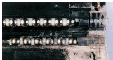
Large amount of foreign matter has entered the raceway
