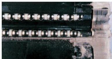
No foreign matter entering the raceway observed
