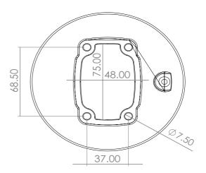
Ø134mm Panel Coupling provides the connection between the operator arm and the operator panel. ARM130.310 is a fixed module. The diameter is 130mm and produced for wide panels with depth.
