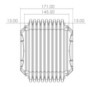
ARM130.505 Steel Interconnection Module - With Bellows is used to mount two operator arms to the connection points horizontally enabling them to move at 90° to the right or 90° to the left. The cast steel body of this product safely combines heavy and long arm configurations.
