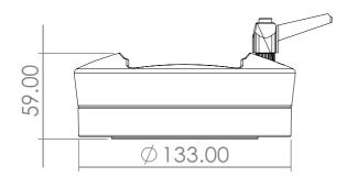
ARM130.320 Rotatable Panel Coupling provides the connection between the operator arm and the operator panel. The diameter is 133mm with a rotation capacity of 315° allowing the operator to rotate the panel to any desired position. It is produced for panel types with high depth ratio.
