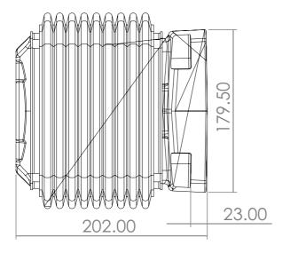
The Steel Wall-Mounted Module - With Bellows helps fixing the operator arms horizontally which are positioned on vertical surfaces. This product with its cast steel body gives reliability for heavy loads and long-distance arm configurations. It allows a mobility of 90° to the right and left.
