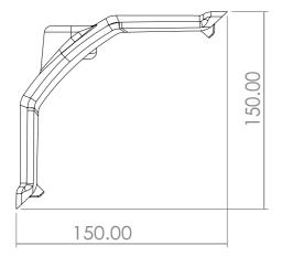
ARM130.811 Warning Lamp Cover (M18) is placed on the corner module ensuring an area for the warning lamp to be placed. The warning lamp connection diameter is M18×1.5
