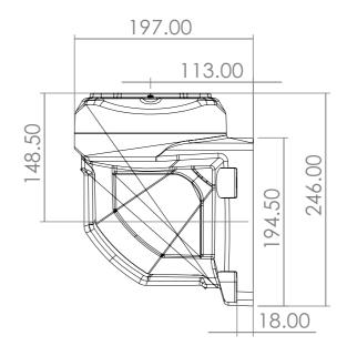
ARM130.710 Rotatable Wall-Mounted Hinge Vertical Outlet is designed to create a connection point to any preferred point vertically. It allows the operator arm to move at a 315° left and right fo heavy loads configurations.
