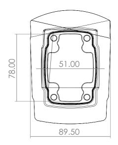
130/080 Support Arm Adaptor is used to secure the connection between ARM130 and ARM080 Its is designed for configurations of heavy loads. The configurations with this product prevent vibrating and sagging as a result of heavy loads. This support Arm Adaptor can be used horizontally or vertically.
