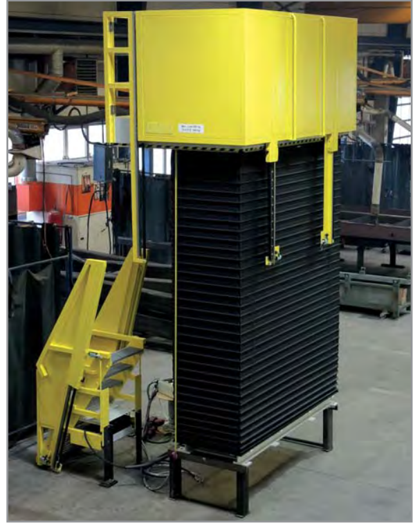
Bellows for elevating platform
