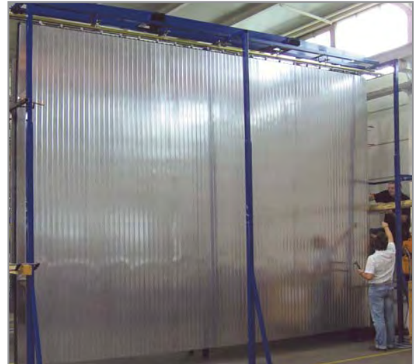
Venetian blind type cover with SAMURAI Bellows for moving column machine
