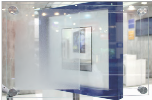
Comparison of glass pane without/with PERLUCOR after sandblasting
