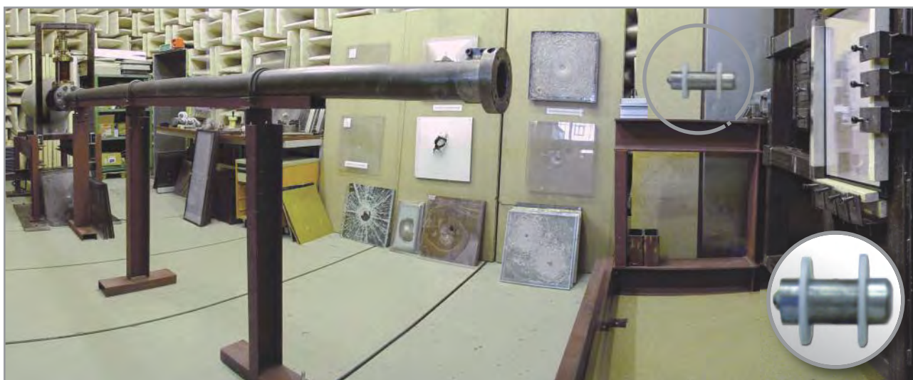
Panorama view of test laboratory at the IWF of TU Berlin. In the foreground acceleration pipe with projectile (eniarged).
